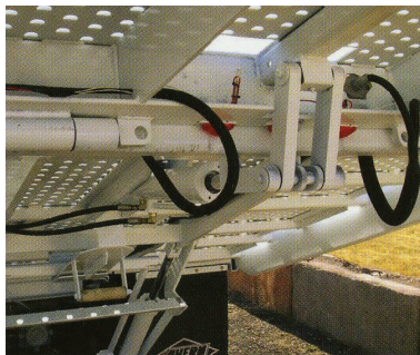
Underside of lift flip tail controlled by hydraulic cylinders
